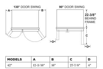
Allow minimum clearances for Freezer door (Dimension A) and Fresh Food door (Dimension B) for a full  $130^{\circ}$  door swing and to allow for drawer removal.
