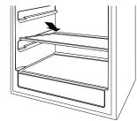
Place in slots when replacing the shelf
