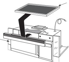
Filter Kit JX81H– Recirculating Charcoal Filter Kit To be used when the Spacemaker microwave oven cannot be vented to the outside.
