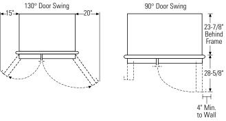
Allow minimum clearances for freezer door and fresh food door for a full 130° door swing and to allow for pan removal.
