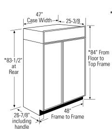
\* Shipping height. The refrigerator can be adjusted to fit into a cutout that is 83-1/2" min. to 84-1/2" max. height Note that the top case trim at the front is 1/2" higher and will overlap upper cabinetry or soffit. Use leveling leas and wheels for a maximum 1" height adjustment.
