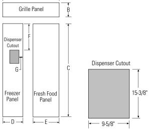
\*Cut the dispenser opening after the backer, spacer and overlay panels have been assembled.
