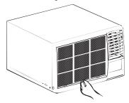
Remove the two grille frame screws.
