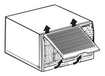
Using the tab, pull up slightly on the filter to release it and pull it down to remove.
