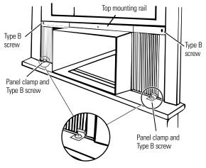
NOTE: Seal any openings around the case or accordion panels with sealer or foam gaskets.
