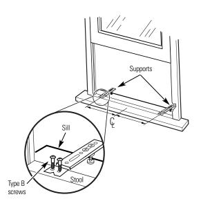
Adjust the leveling bolts against the sill so that the supports have a slight tilt to the outside. Use a level; about 1/2 bubble will be the correct slant to the outside.
