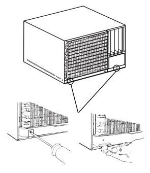
Remove the screw securing the ground wire to G the right side face of the unit.
