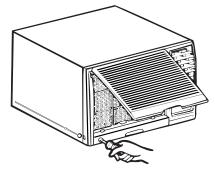
Install the filter. Hook the inlet grille in the frame and close it. Connect power.
