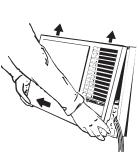
Remove the two locking screws and locking brackets from the lower front of the unit.
