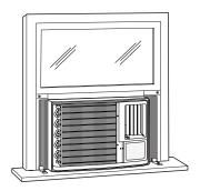
**B** Reinstall the locking brackets and screws removed earlier.
