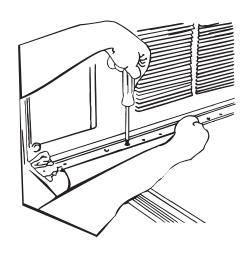
Extend the left and right accordion panels to the vertical window sashes, drill 1/8" pilot holes, and attach the top corners with 2 Type B screws. Use an accordion panel clamp on each lower corner to trap the panels. Drill 1/8" pilot holes and attach the panel clamps with Type B screws.
