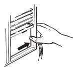
Push the grille to the left and raise it up. Lift the grille frame up and off.
