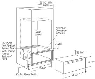
Note: Additional clearance between cutouts may be required. Check to be sure that oven supports above the Warming Drawer location do not obstruct the required interior 23-1/2" depth and 9-1/4" height.
