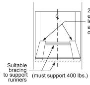
2 x 4 or equivalent runners level with bottom of cutout and flush with sides of cutout or solid bottom floor.
