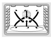
In a convection oven, a fan circulates hot air over, under and around the food.
