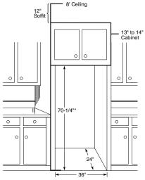
"The rough-in dimension of 70-1/4" is minimum and is measured from the finished floor to top of opening (or the underside of the overhead cabinets). For Models with Trim Kit: If trameless style cabinets are planned for above the retrigerator, you may need to consider adding a maximum of 14" (70-1/2") to height of opening to allow additional clearance between cabinet doors and top of refrigerator trim when cabinet doors are in open position.
