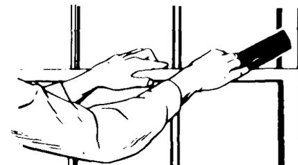
1. Slide the chassis into the installed cabinet (provided with AJK models) or wall sleeve RAB36, RAB37 or RAB38 (not provided) designed for AJJ models. Make sure that the tubing on the unit is not touching the wall case and that the wall case insulation is secure.
