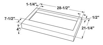
A stainless steel liner is shipped with each hood insert. This non-combustible liner protects the underside of the canopy.
