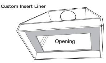
The custom canopy must be sized to fit the insert sleeve. Construct the canopy with an opening that is:  $26"W \times 13-3/16"D$  The opening must be constructed of 3/4" thick material to allow the sleeve locking clips to engage.
