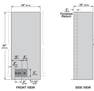
**NOTE:** GFI (ground fault interrupter) is not recommended. Water line can enter the opening through the floor or rear wall. The water line installed should be 1/4" O.D. copper tubing or GE SmartConnect™ tubing between the cold water line and water connection location. The line should be long enough to extend to the front of the refrigerator. Installation of an easily-accessible shutoff valve in the water line is required.
