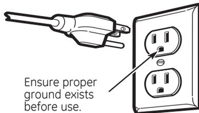
Where a standard two-prong wall receptacle is encountered, it is very important to have it replaced with a properly grounded three-prong wall receptacle, installed by a qualified electrician.
