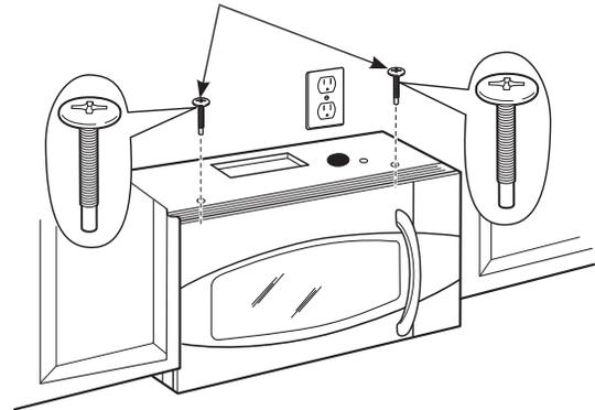
**5** Tighten the outer two screws to the top of the oven. (While tightening screws, hold the oven in place against the wall and the top cabinet.)
