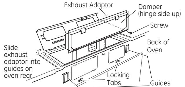
Push down securely until it is in the lower locking tabs. Take care to assure the damper hinge is installed so that it is at the top and that the damper swings freely.
