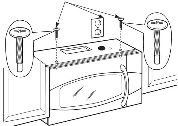
**6** Tighten the outer two screws to the top of the oven. (While tightening screws, hold the oven in place against the wall and the top cabinet.)
