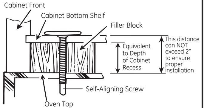
**4** Insert 2 self-aligning screws ( $\frac{1}{4}$ "-28 x  $2\frac{5}{8}$ ") through outer top cabinet holes. Turn two full turns on each screw.
