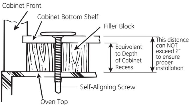
5 Tighten the outer two screws to the top of the oven. (While tightening screws, hold the oven in place against the wall and the top cabinet.)
