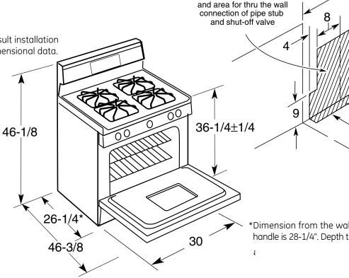
Recommended area for 120V outlet on rear wall
